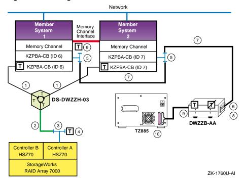
Table 8–6 shows the components used to create the cluster shown in Figure 8–7.
